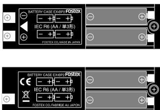
**<Note>**: Always use eight new alkaline or fully charged nickel hydride batteries of the same model and same capacity.
