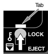
**<Memo>**: To remove the battery box, slide down the [EJECT/LOCK] lever to unlock the battery box. The battery box is slid to the front a few millimeters and you can pull it out by hand.
