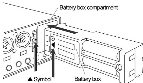
After fully inserting the battery box, slide up the [EJECT/LOCK] lever to the LOCK position. A tab appears as shown on the right figure and the battery box is locked.
