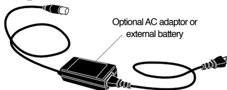
**<Note>**: The rated voltage of the [DC IN] connector is DC 10 V to 24 V. When you connect an external power source to the [DC IN] connector, use the appropriate power source that matches the rated voltage of the [DC IN] connector. For the detail information on the pin assignment of the [DC IN] connector, see page 12 of "Features and controls".
