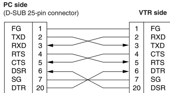
Using crossover cable with D-SUB 9-pin and 25-pin connectors
