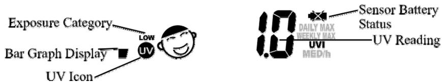
To access UV mode from the main unit press **UP** or **DOWN** until the UV icon
