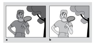
Turn on Backlight Compensation by pressing the Backlight Compensation button (♣).
