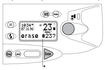
4 To erase the picture, press the Erase button a second time. (If you decide not to erase the picture, do **not** press the Erase button. Instead, wait for the confirmation message to disappear or press the Enter button.)
