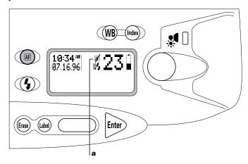
You can reset to Auto Focus On (\*\*E\*) by pressing the Auto Focus button again. The camera automatically resets to Auto Focus On when the camera is turned on.
