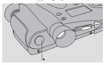
2 Unlatch and remove the PDC-2000 battery holder from the camera.
