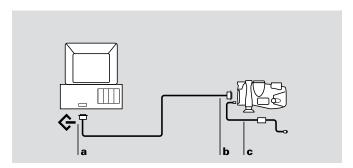
Use only the SCSI cable provided with the camera. Other cables may appear similar, but could damage the camera or your computer.
