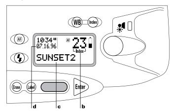
3 Simultaneously press and release the Erase button and the Shutter button to display a confirmation message (e) on the LCD panel. (Be sure to press the Shutter button all the way.)
