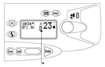
A symbol (\*\*) in the LCD panel (a) indicates that Backlight Compensation is on. The camera automatically turns Backlight Compensation off after you take a picture or when the camera is turned on.
