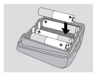
6 Insert the battery holder in the camera and close it, making sure it latches.
