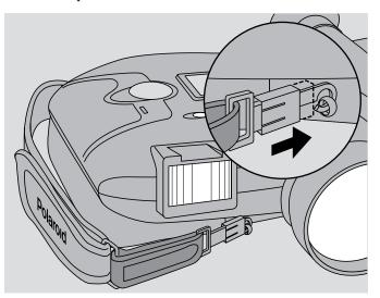
To attach the shoulder strap, connect the ends of the strap to the eyelets on the back of the camera as shown. Be sure to slide the plastic sleeve on each hook toward the eyelet until it snaps, locking the strap securely.
