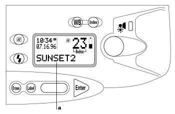
With the procedures in this section, you can edit the default picture label applied to all pictures taken after the default label is entered. (Your PDC-2000 camera was shipped with "POLAROID" as the default picture label.) You can also edit this default label to create unique labels for individual pictures any time after the pictures are taken.
