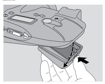
2 Unwrap and install the four "AA" NiCad batteries provided, observing the battery orientation label in the battery holder. (Install the two outside batteries first, then install the two inside batteries.)
