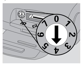
3 Insert a small screwdriver into the slot and rotate the selector until the arrow points to the desired SCSI ID.
