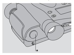
If the PDC-2000 is the only SCSI device If the PDC-2000 camera is the only external SCSI device being used with your computer, turn off the computer and the camera. Then connect the SCSI system cable provided to the computer's SCSI port (a). Connect the other end of the system cable (b) to the camera's SCSI connector.
