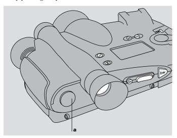
2 Open the connector cover and locate the SCSI ID selector.
