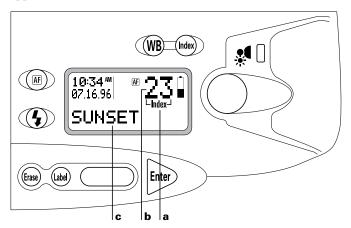
2 If the number (**b**) of the picture receiving the new label is not displayed in the LCD panel, press the Scroll button until the desired picture number and label (**c**) appear.
