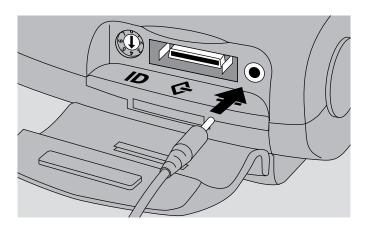
Charge the batteries completely by leaving the charger connected to the camera for about 6 hours (12 hours for new batteries). You can use the camera while the batteries are charging.
