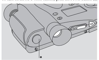
When you press the Power button, the camera performs a brief self-test, then displays a normal LCD panel. If the sound indicators are enabled, the camera also emits a short, high-pitched tone to indicate that it passed the self-test and is ready to take pictures.
