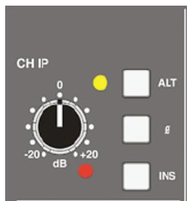
Each one of the 8 mono channel inputs (**CH IP**) on the X-Panda has a choice of two Line Inputs. The first input is traditionally sourced from the Output of a microphone pre amplifier, D.I box or perhaps even a line level instrument. These connections are labelled “**LINE IN 9-16 (1-8)**” on the rear of the desk. They are so labelled due to the fact that you may be using X-Panda stand alone or in conjunction with an X-Desk or indeed additional audio equipment.
