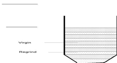
c.) Setting 5 = 10 switching cycles per conveying cycle
