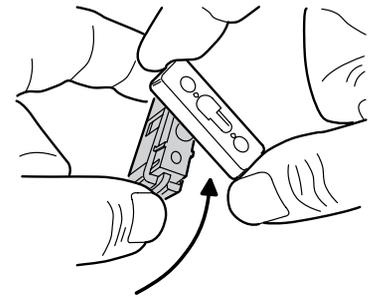
THE SNAP-ON MAGNET SPACER CAN BE USED TO ADD 1/4" HEIGHT TO THE MAGNET (SPACERS CAN ALSO BE SNAPPED TOGETHER FOR MORE LIFT)
