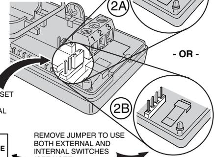
THIS IS THE FACTORY SET JUMPER POSITION, IT SELECTS THE INTERNAL CONTACTS
