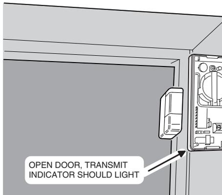
NOTE: THE TRANSMIT INDICATOR WILL ONLY LIGHT DURING TRANSMISSIONS WHEN THE CASE IS OPEN (EXCEPT WHEN PUSHING THE CASE FOR TESTING)
