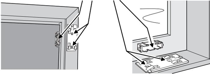
**NOTE: ATTACHING THE TRANSMITTER WITH DOUBLE-STICK TAPE IS NOT ALLOWED IN UL INSTALLATIONS**
