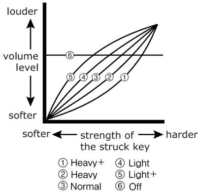
This parameter adjusts the touch response curve of the keyboard.
