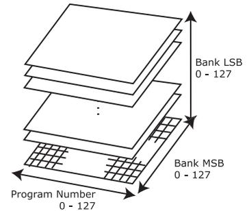
This is a 3D image of the expanded program change system with the MSB and LSB. To use these efficiently and correctly, refer to the operation manual of any external MIDI sound modules that are connected to the MP5.
