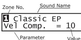
Zone parameters can be edited individually for each zone. There are two parameter groups, Internal parameter group and External parameter group. If a zone is set to Int, only Internal parameters are available for editing. If a zone is set to Ext, only External parameters are available for editing. If a zone is set to Both, both Internal and External parameters are available for editing.
