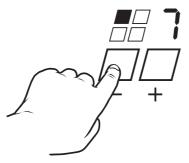
During automatic operation an "A" lights up in the display alternately with the selected cooking setting.
