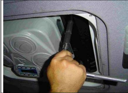
16. Fix the nuts by means of the deep socket spanner. This has to be done evenly.
