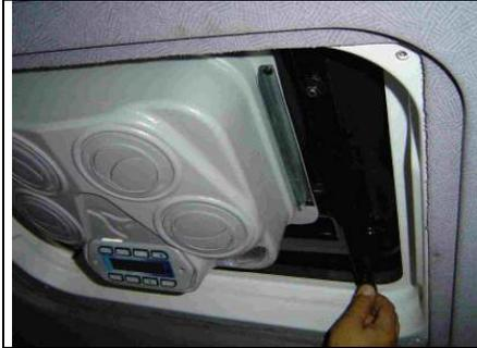
15. Place the fixing strips on the left and right side and turn the nuts carefully without moving the system.
