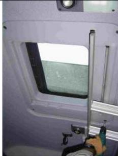
3. Remove the screws, which can be found on the angles of the cover plate round the hatch. Put the cover plate on a place where it cannot be damaged
