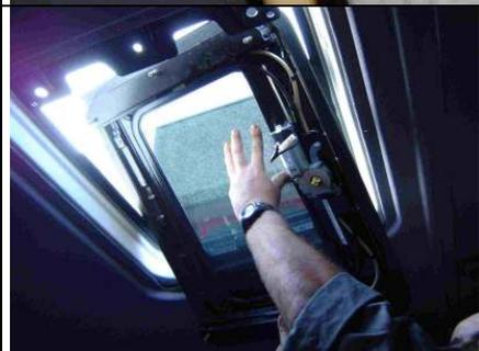
6. Remove the hatch by pulling it diagonal inside. Put the hatch on a place where this cannot be damaged
