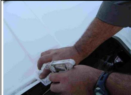
9. Moisten a cloth with an alcohol solution or an other degreasing solution and clean the edge on the roof all around. Don't spray, in case you damage the interior
