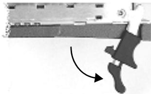
**Lever Fully Open** - Pull the lever handle(s) to a fully open position (approx. 70 degrees), as shown here
