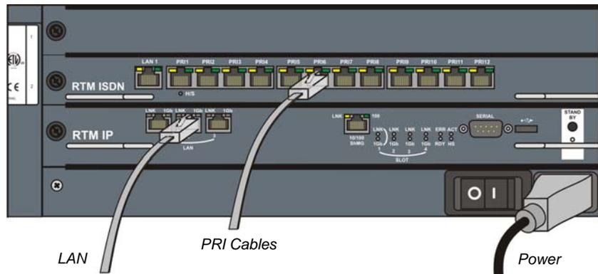
7 E1 or 9 T1 cables can be connected to each RTM ISDN card, up to a total of 14 E1 or 18 T1 PRI cables when two RTM ISDN cards are installed.
