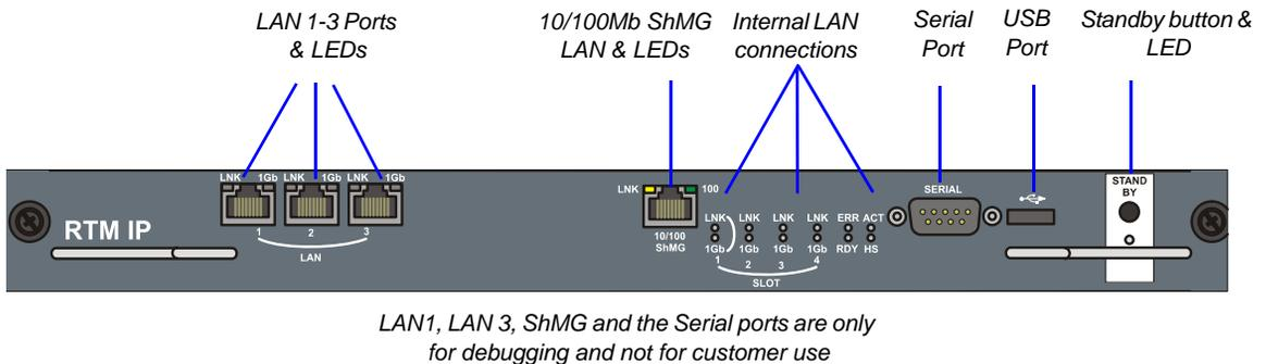
**Figure 1-2** RMX 2000 RTM IP Rear Panel Layout
