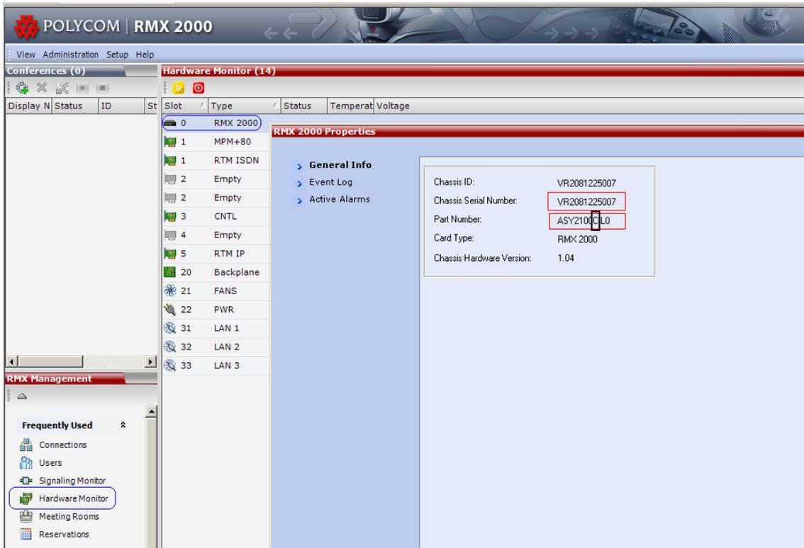
The RMX Part Number contains the letter A/B/C/D that represents the chassis type, as shown in the capture above.
