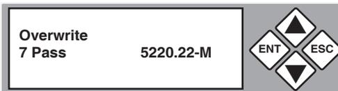
This method will write over the entire capacity of the hard drives connected to the 1:5 HDD Cruiser seven different times.
