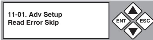
3. Press **ENT** to display the current configuration setting. The default setting is “Off”.
