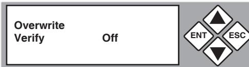
Use the arrow buttons to toggle between “On” and “Off”. Press **ENT** to select.
