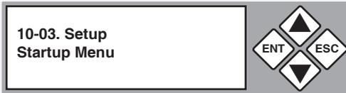
3. Press **ENT** to display the current configuration setting. The default setting is “1. Copy HDD”.
