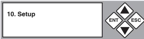
2. Use the arrow buttons (▼▲) to toggle between the subfunctions. Press **ENT** to select “Startup Menu”. The following screen will be displayed.
