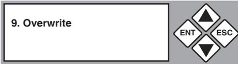
**Note:** Overwriting the entire capacity of all connected hard drives can take an extended period of time.
