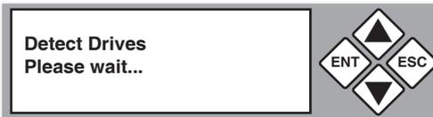
During the PreScan process, the 1:5 HDD Cruiser will display progress information.
