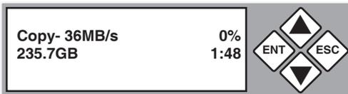
The amount of data remaining to be transferred (shown in gigabytes), and time will be displayed as the percentage of completion increases.
