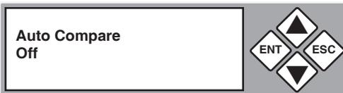
4. Use the arrow buttons (▼▲) to modify the setting. After you change a setting, remember to press **ENT** to save it.
