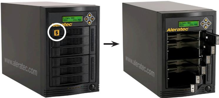
2. Take the Hard Disc Drive (HDD) and align the drive's SATA plug to the lower right hand side of the drive bay.
