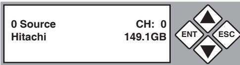
4. Use the arrow buttons (▼ or ▲) to show information about any additional hard drive that is connected. The following screen will be displayed.
