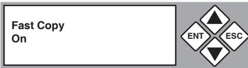
4. Use the arrow buttons (▼ or ▲) to toggle between “On” and “Off”. Once you change a default, remember to press **ENT** to save it.
