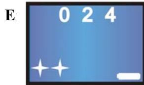
Press the Shutter button within 5 seconds to change the resolution setting on your camera. The resolution will be changed, and the camera will automatically revert to Preview mode
