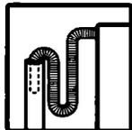
Is the drain hose lower than the water level in the washer? It must be higher.
