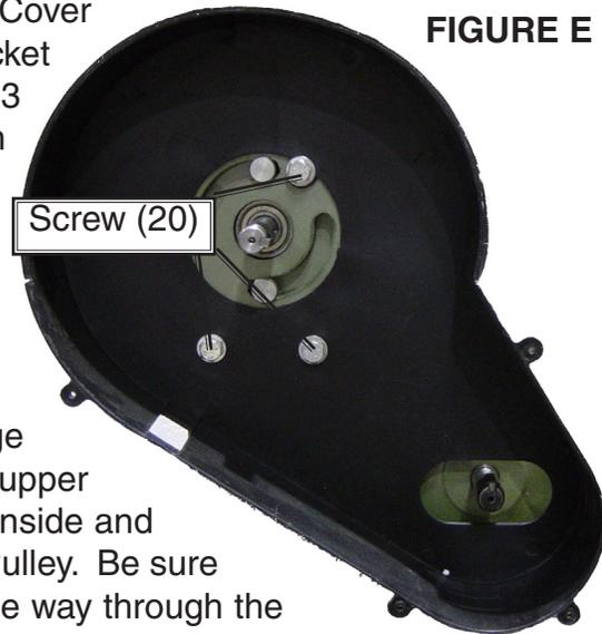
3. This item is packed with tape on the shafts to keep the keys in place. Remove the tape from the upper shaft, being careful to not lose the key.
