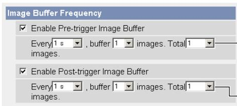
(B) The number of [Enable Pre-trigger Image Buffer] images (B) must follow:  $(B) < (A) \times 1/3$
