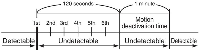
A Motion Detection signal is detected.
