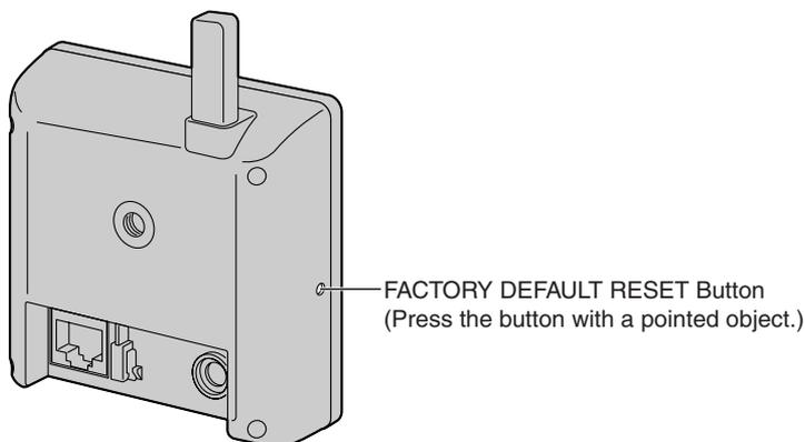
Pressing the FACTORY DEFAULT RESET button resets the camera to factory default. If you lose your user name and password, use this button to reset the camera. To restore the wireless connection, access the camera by using a wired connection and set up the wireless configuration. (For BL-C20A, see Getting Started.)
