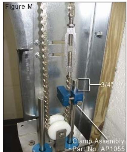
Rod with turnbuckle (Part No. CL100 and CL101) will rise when opening the door
