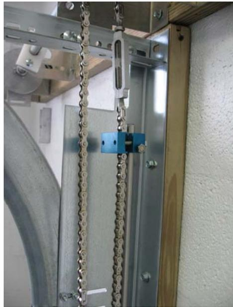
Now attach Part No. 'CL102' to the rod that is not extended out of the cylinder
