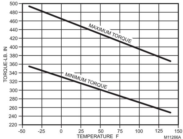
**Fig. 1. Minimum and maximum torque versus temperature.**
