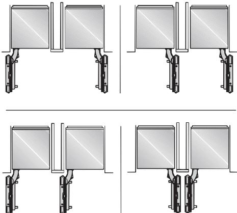
If there is a partition with a thickness **from  $\frac{5}{8}$ " (16 mm) to  $6 \frac{5}{16}$ " (160 mm)** between the adjacent appliances, then each appliance should be individually installed within its own niche using the mounting accessories included. The "Merging Kit" will also be needed.
