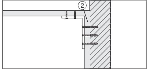
Two anti-tip brackets are recommended for each appliance. For side-by-side installations 4 brackets are recommended.
