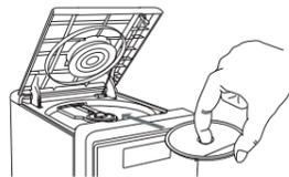
4. Press the CD compartment lid (OPEN/CLOSE portion) again to close it. "READING" blinks for several seconds, then the total number of tracks and total playing time appear.
