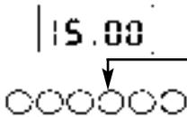
**Step 2** Press the Manual button to return the oven(s) to "Manual" operation. The 'Auto' symbol will go out.
