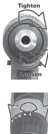
Twist the 24 setting torque control ring to the desired setting. Lower settings are better for light work such as driving screws into soft materials. Higher settings are recommended for drilling into harder surfaces.
