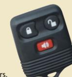
Press this control once to lock all doors. Pressing the control a second time will chirp the horn and flash the lights to confirm that all doors are closed and locked.
