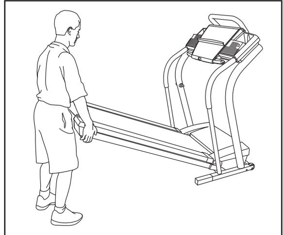
2. Move your right hand to the position shown and hold the treadmill firmly. Using your left hand, pull the latch knob to the left and hold it. Raise the treadmill until the latch pin is aligned with the indicated hole in the side of the treadmill. Insert the latch pin into the hole. **Make sure that the latch pin is fully inserted into the hole.**
