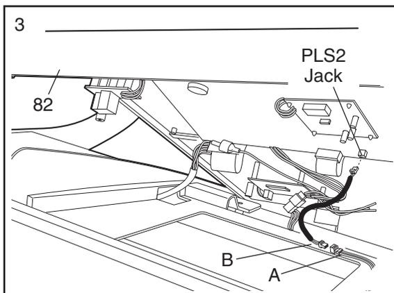
**Make sure that no wires are pinched.** See step 1. Reattach the Console (82), **making sure that the screws are inserted into the same holes from which they were removed.** See step 6. Reattach the Upper Handrail (122).
