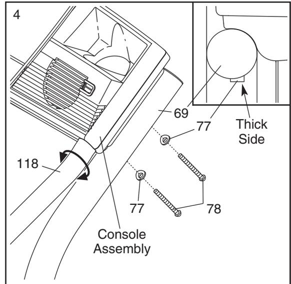
Next, lift the console assembly and the Handrail (118) slightly and align the 4 1/2" Bolts (78) with the holes in the Handrail. Thread the Bolts into the Upright (69) and the Handrail until the heads of the Bolts are against the Upright. **Do not tighten the Bolts yet.**
