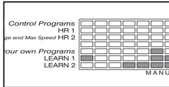
For about six seconds after a program is selected, the Incline/Heart Rate display will flash the maximum incline setting for the program, and the Speed display will flash the maximum speed setting for the program. The Time/Pace display will show how long the program will last. The program display will show the first ten speed settings for the program. **Note: If only three columns of indicators are lit in the program display, see HOW TO CREATE A CUSTOM PROGRAM on page 15.**
