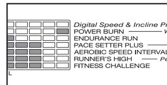
For about six seconds after a program is selected, the Incline/Heart Rate display will flash the maximum incline setting for the program, and the Speed display will flash the maximum speed setting for the program. The Time/Pace display will show how long the program will last. The program display will show the first ten speed settings for the program.
