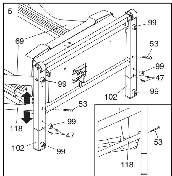
Attach each Extension Leg (102) with two 1" Tek Screws (47) and a Base Pad (99) as shown. (Note: Attach the lower Screw, without the Base Pad, first.) Next, align the lower ends of the Handrails (118) with the holes in the base of the Uprights (69). Attach each Handrail with a 4" Bolt (53) as shown. **Note: The Bolts must be at an angle that matches the angle of the Handrails as shown in the inset drawing.**
