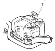
WARNING! If the idle speed cannot be adjusted so that the cutting attachment stops, contact your dealer/service workshop. Do not use the machine until it has been correctly adjusted or repaired.
