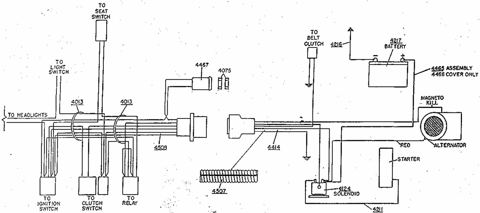
BODY WIRING LOOM - 4508
