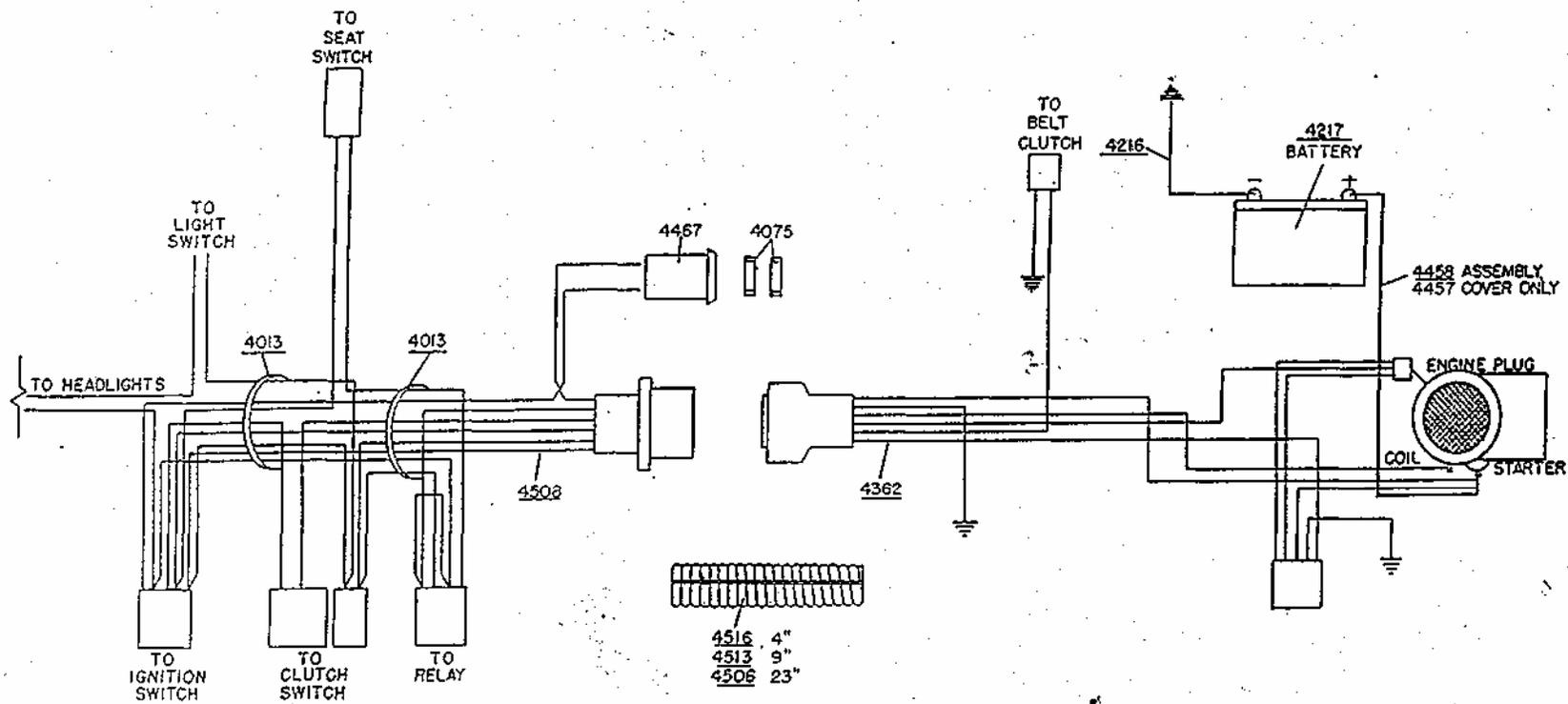
BODY WIRING LOOM - 4508
