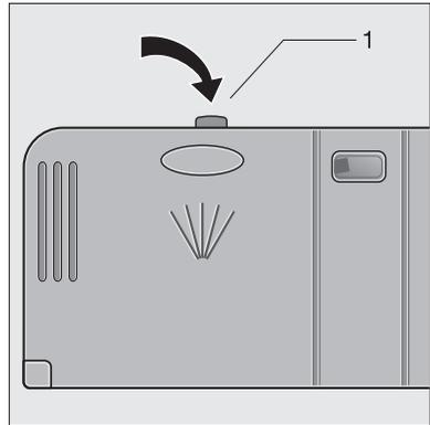
2. Fill the detergent dispenser with detergent. The markings indicate the dosing levels: "20" corresponds to approx. 20 ml of detergent, "30" corresponds to approx. 30 ml of detergent.
