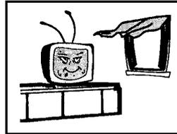
Do not cover the Ventilating holes in the cabinet. Keep a space of more than 5cm from the walls to the TV set, to guarantee the good ventilation.
