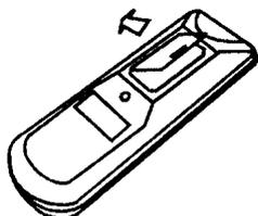
(2) Insert two size AAA batteries according to the polarity indication inside the remote controller.
