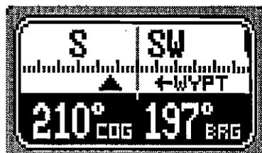
When a waypoint is recalled (see the waypoint navigation section), the direction to the waypoint, or bearing, is shown in the bottom right corner of this box (BRG).
