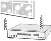
If it is very cold, please turn on the power for 1min. Then turn off the power for 1 min. Then you can turn on and use the unit
