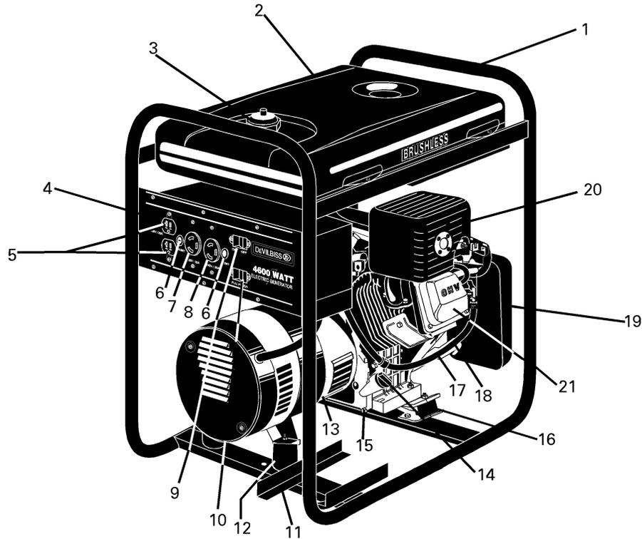
1. **Frame assembly**- Protects generator and engine as well as a means to handle complete unit.
