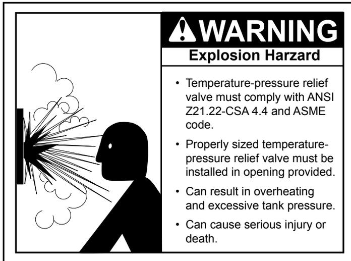
Manually operate the temperature and pressure relief valve at least once a year to make sure it is working
