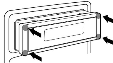
⚠ To attach this unit, make sure the front of the control panel faces you and fit it into the mounting sleeve by pressing the four corners of the hard rubber frame at the same time. Do not apply strong pressure to other sections than the corners; otherwise troubles such as the impossibility of opening or closing the panel may result.
