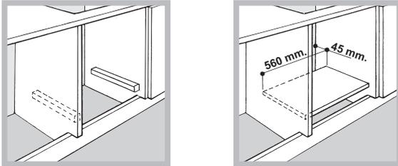
! The hob can only be installed above built-in ovens with a cooling ventilation system.
