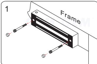
1 Tighten the electromagnetic lock on the L bracket by using the fixing screw.
