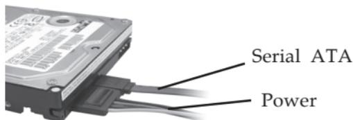
Figure 2: SATA hard disk drive connections
