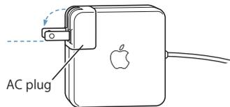
**Important:** Be sure to snap the electrical prongs on your AC plug into their completely extended position before you plug the adapter into the outlet.
