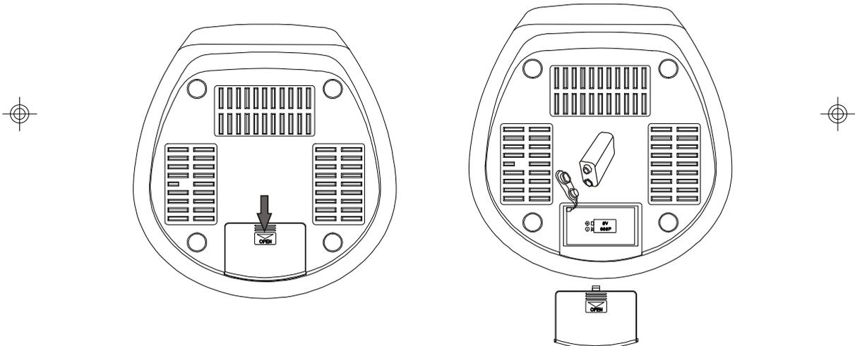
If the power is interrupted the clock display will go off but the battery will maintain the clock and alarm time settings. When power is restored the time display will be correct and your alarm setting will also be maintained.
