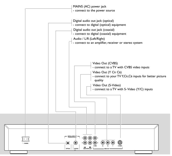
Caution: Do not touch the inner pins of the jacks on the rear panel connectors. Electrostatic discharge may cause permanent damage to the unit.
