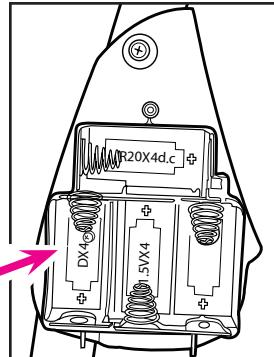
**With baby out of swing,** open the battery compartment lid by unfastening screw. Insert four "D"-LR20 (1.5V) batteries. Replace battery lid.
