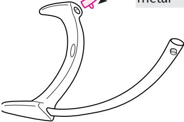
Push front leg tubes into crossbrace until the metal buttons snap inside the crossbrace.
