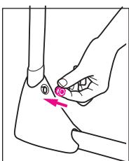
Secure foot with nut and bolt.
