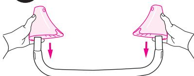
Place feet on "U"-shaped tube as shown.
