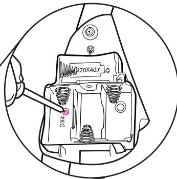
Insert screw into hole to secure the other leg. Replace lid.
