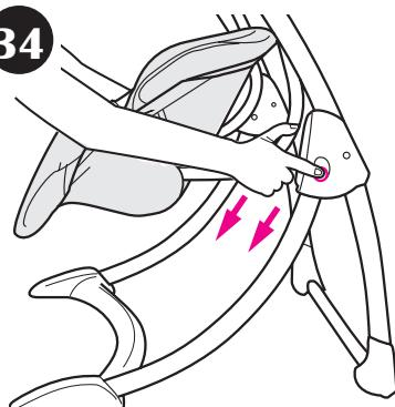
Press buttons on each side of swing to remove front legs for storage.
