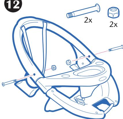
Insert screws exactly as shown with nuts on the inside of frame. Tighten screws.
