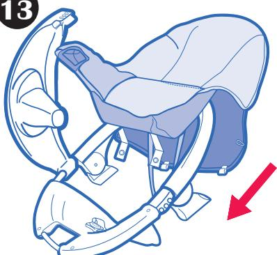
Open tray and slide seat pad over frame as shown.
