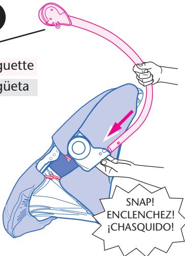
Snap swing arm into opening on bracket. Repeat on other side. Tab at top of arm must face away from seat.
