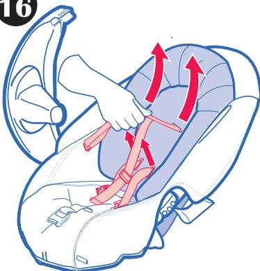
Attach head support by pulling the shoulder straps and waist straps through the holes as shown.
