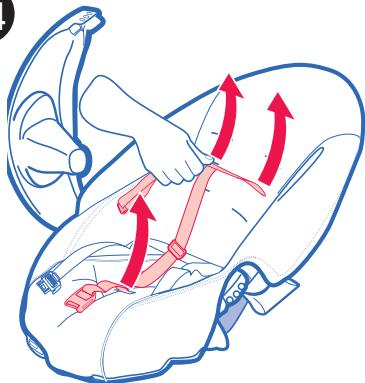
Pull the crotch strap and the shoulder straps through seat pad as shown.
