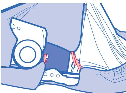
Make sure all 6 straps are attached. There are 3 on each side of the unit.
