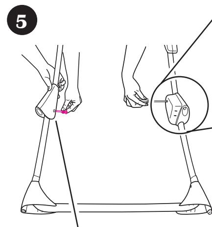
Secure leg and arm connector with screw.
