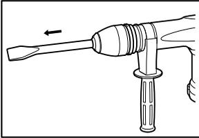
To remove the bit, pull the chuck cover down all the way and pull the bit out.
