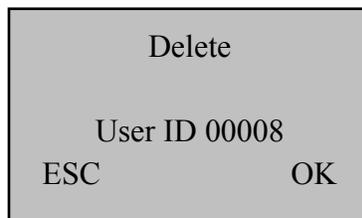
**Note: You cannot delete a user with multiple enrolled fingerprints without deleting each fingerprint first. If the user has a password you will also need to delete it before you can remove the user from the terminal.**
