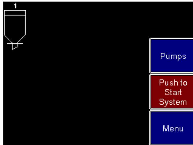
1. At the “Station Status” screen (Figure 2) or at the “Pump Status” screen, touch the **Menu** button. The “Menu” screen opens.
