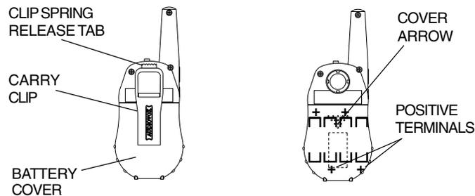
1. Using thumb, press down on battery cover at arrow and slide cover down.
