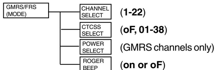
**NOTE:** To differentiate between operating modes, look for **HI** or **LO** indication below the battery power level indicator when in GMRS mode. Refer to the appropriate section of this manual for detailed operating instructions for each mode. Channels 1 through 7 are shared GMRS/FRS. Channels 8 through 14 are FRS only, and channels 15 through 22 are GMRS only.
