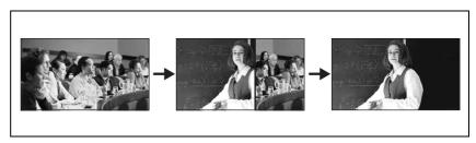
Each time you press the AUTO TRANS button or move the transition lever, the program output video is switched to the video selected with the NEXT select button in a wipe transition.
