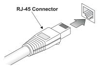
Figure 3-1 RJ-45 Connections
