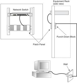
Figure 4-2 Wiring Closet Connections
