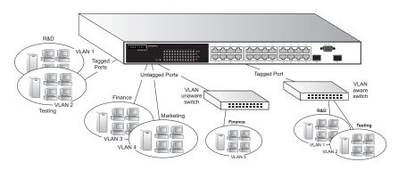
Figure 2-4 Making VLAN Connections
