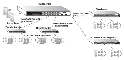
Figure 2-3 Remote Connections with Fiber Cable
