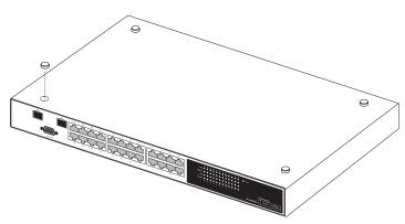
Figure 3-4 Attaching the Adhesive Feet
