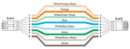
Figure B-2 Straight-through Wiring
