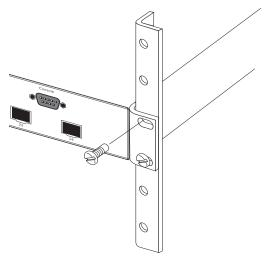
Figure 3-3 Installing the Switch in a Rack
