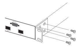
Figure 3-2 Attaching the Brackets
