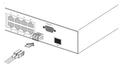
Figure 4-3 Making Connections to SFP Transceivers
