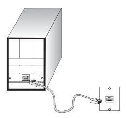
Figure 4-1 Making Twisted-Pair Connections
