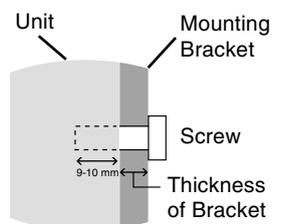
Screw length should equal depth of hole (9-10 mm) + the thickness of mounting bracket.
