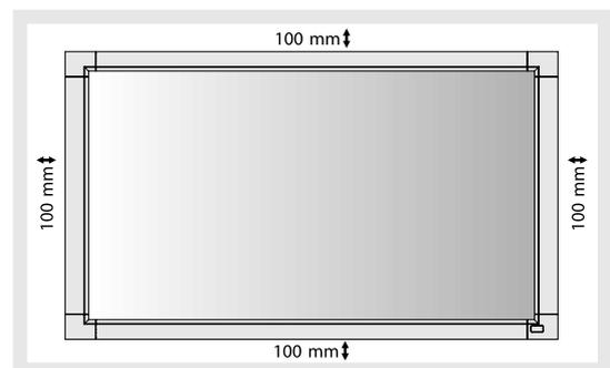
Allow adequate ventilation or provide air conditioning around the monitor, so that heat can properly dissipate away from the unit and mounting apparatus; especially when you use monitors in a multiple screen environment.
