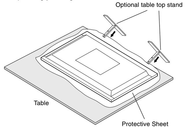
**NOTE:** ST-3215 is for V321. Use the Thumbscrews included with ST-3215. ST-4020 is for V461 and LCD4215<sup>(R)</sup>. (V461 and LCD4215<sup>(R)</sup> are not mentioned in ST-4020 manual). Before using optional table top stand, remove installed thumbscrews from the display first. Please use a screwdriver for removing thumbscrews as necessary.
