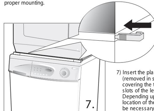
7) Insert the plastic covers (removed in section 2) covering the two front slots of the leveling legs. Depending upon the location of the unit, it may be necessary to change the side on which the dryer door opens.
