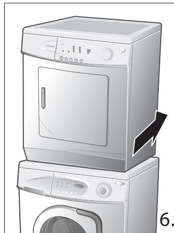
6) Gently push the dryer into position as indicated in figure 5 & 6, sliding the unit into the slots provided. It is important that the dryer is level. Make sure all four leveling legs are pushed all the way back into the slots to ensure proper mounting.
