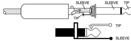
1/4" TS Unbalanced Wiring:
