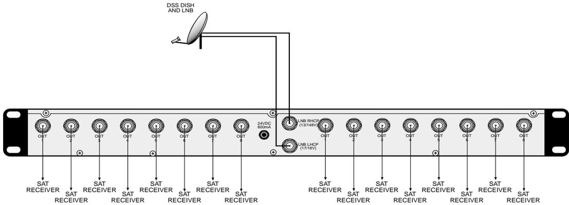
1. Connect the RHCP LNB output and the LHCP LNB output to the RHCP(13/14V) and LHCP(17/18V) inputs respectively of the TSMS-2150X-16A.
